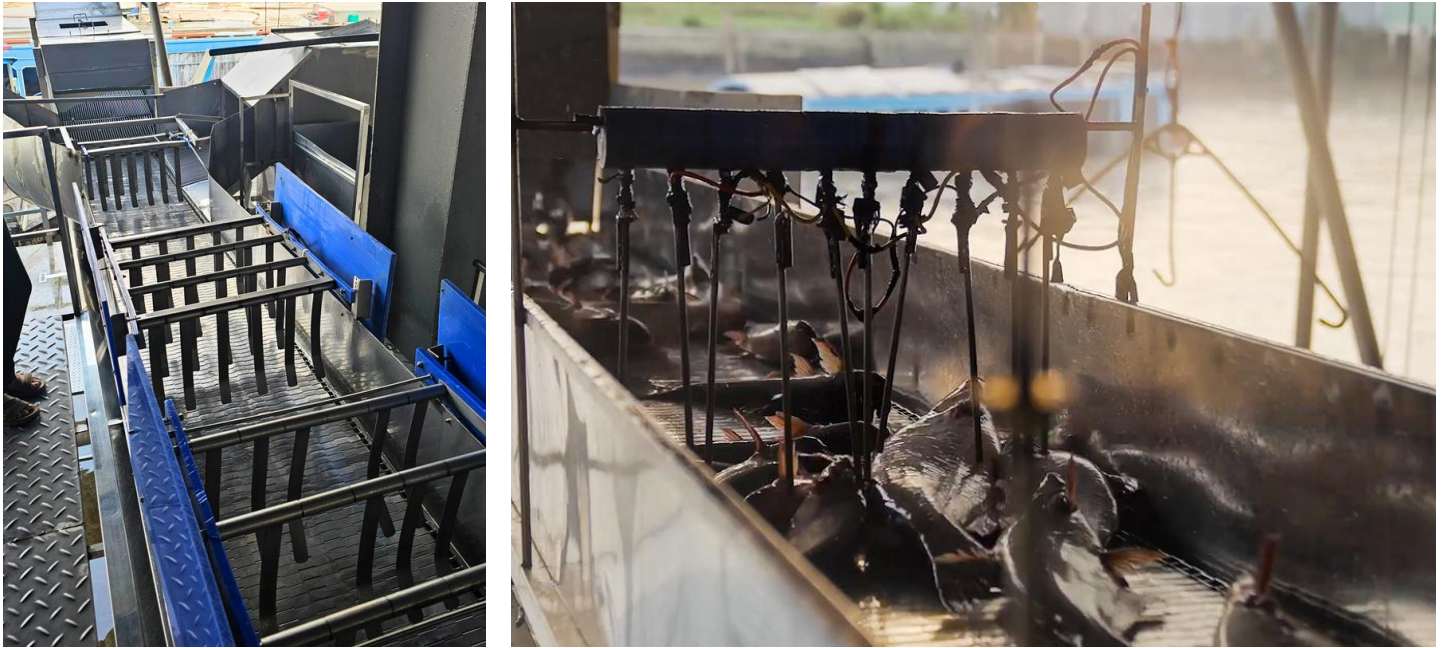
Figure 19. House-made dry stunner at one processing facility. Out of operation (left) and in operation (right). Right picture © Pham Cong 34 .
